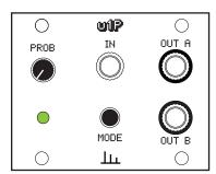
The u1P is a Bernoulli gate. Based on the probability set by the potentiometer, it routes a trigger signal sensed at the input to either of its two outputs. Press the MODE button to alternate between updating the output at both rise/fall edges or only at rise edge. Press and keep holding the MODE button to change modes: the potentiometer determines the selected
