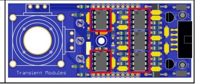
19. Place the 2x **10 pin male header** and solder both ensuring they are 90° to the PCB.
