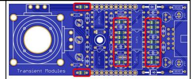
3. Solder the 1x 10K resistor.
