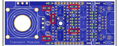
6. Solder the 1x 4K7 resistor.
