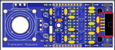
17. Solder the 5x **IC Sockets**. Make sure the **notches** in the sockets match the silkscreen.
