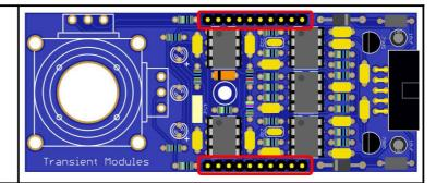
20. Now the top board. Solder the 3 remaining resistors: **1K**, **470K**, **100K**.
