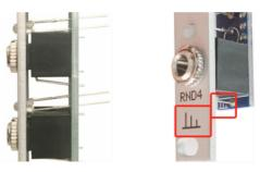
18. Solder all the LEDs and jack sockets and cut **ALL** the legs from **both** LEDs and jack sockets. Also leave the **NORM** SMD jumper **unsoldered** for now (TRIG2 won't be normalized to TRIG1 yet).
