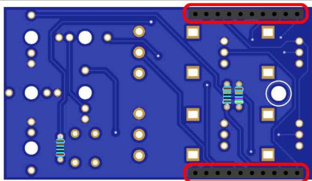
24. Place the 4x **100KB** pots making sure they're **fully inserted**. Also place the 5x **jack sockets** and the 2x **switches**.
